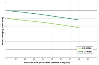
NOTE: Graph shows inlet pressure at a temperature of 20°C (tolerance  $\pm 10\%$ )
